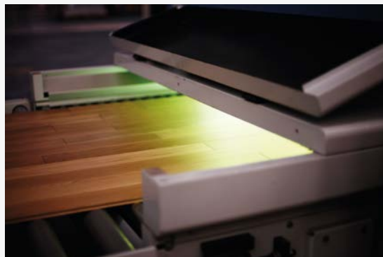
Varnishing process with UV drying.
